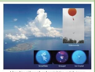
A launching videosonde and precipitation particle images
